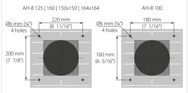
3. Insert the supplied expansion anchors 6 mm (1/4")x40 mm (19/16") into the holes. Disassemble the outer ventilation hood to enable access to the fastening holes. Remove the ventilation hood front part.
